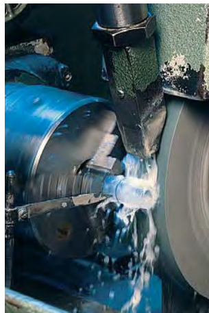
Circular grinding machines grind NS-cones half-automatically
